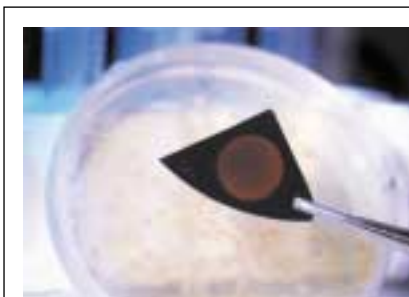
Figure 1. A porous silicon microcavity resonator. The device is used as a biosensor to detect Gram-negative bacteria (shown in the background). Figure kindly supplied by Elizabeth Lamarck, University of Rochester (Rochester, NY, USA).
